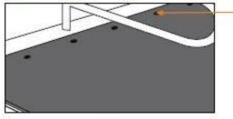
fasten at the front edge through the prefabricated fastening points
